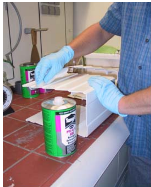
Final cleaning with Tangit-cleaner is done using papertowels (removal of lubricant and partial dissolution of the surfaces).
