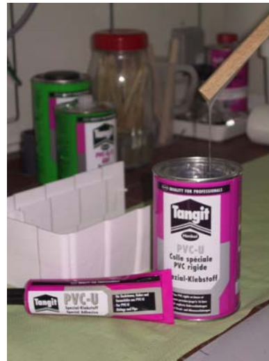
Stir Tangit PVC-U well before use. It should flow slowly off a stick hold at an angle, forming a trail.
